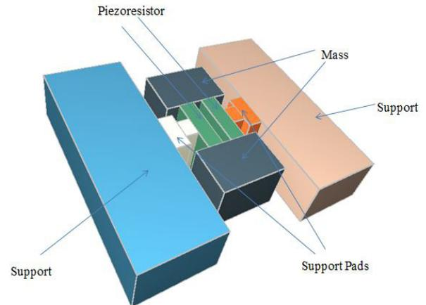
**Figure 1.** 3-D schematic of the dog-bone thermally actuated resonator with piezoresistive readout<sup>12</sup>.
