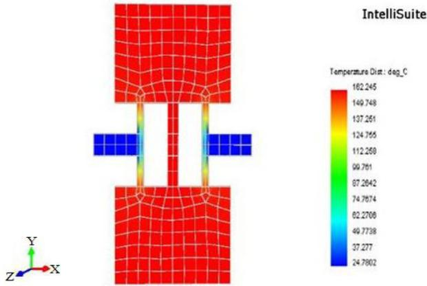
**Figure 5.** Temperature profile of the modified resonator structure.
