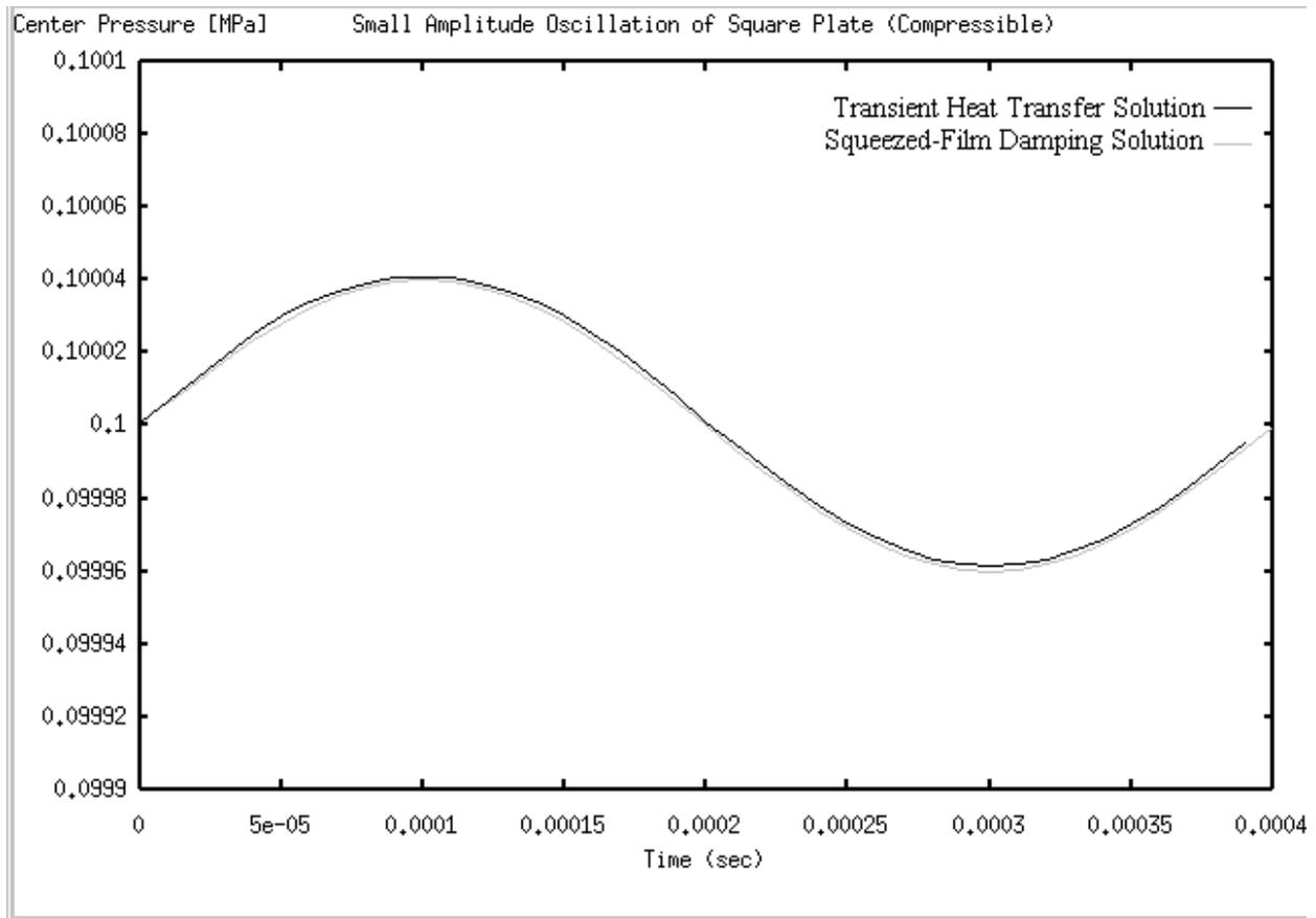
**Figure 8:** Comparison of the time history of pressure at the plate center.
