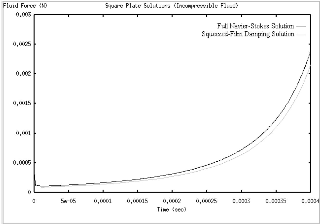
**Figure 4:** Comparison of fluid pressure force on a moving square plate calculated using squeezed-film damping and full Navier-Stokes CFD
