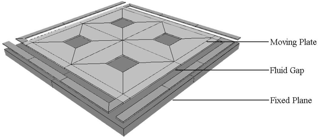
**Figure 1: Porous plate moving relative to a fixed solid surface**
