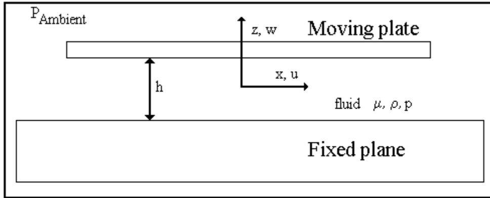
Figure 2: Squeezed film model variables
