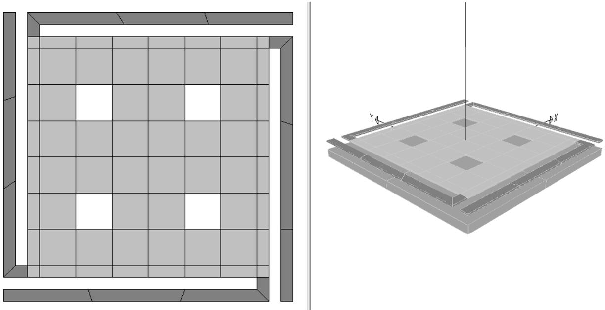
**Figure 5:** Square plate with cutouts moving in incompressible liquid
