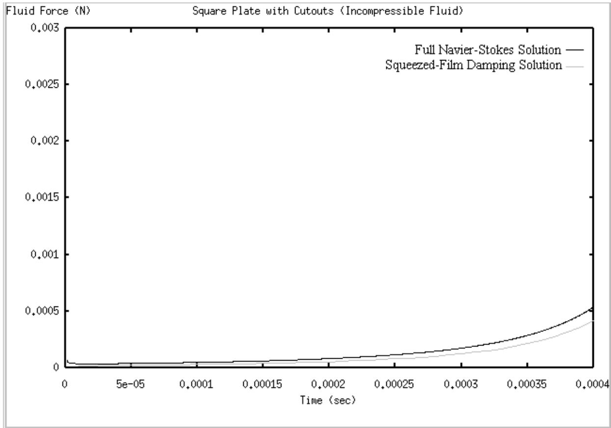
**Figure 6:** Comparison of fluid pressure force on a moving square plate with cutouts calculated using IntelliSuite and full Navier-Stokes CFD
